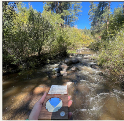
ELLIE USING A DENSIMETER AT BATTLESHIP ROCK
